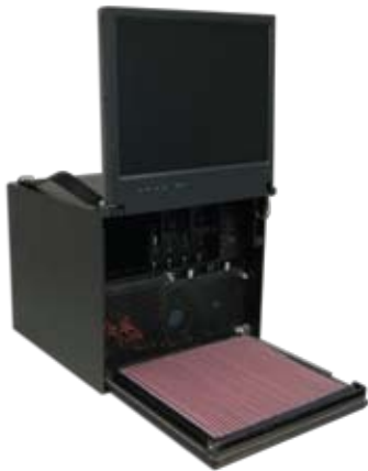
Filter frame and filter folds down revealing all drives
