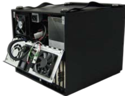
Rear fans fold down allowing inner chassis removal for easy access to all components
